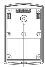
Anti-tamper photocell. To activate the function, please refer to page 16 "Anti-tamper function"
