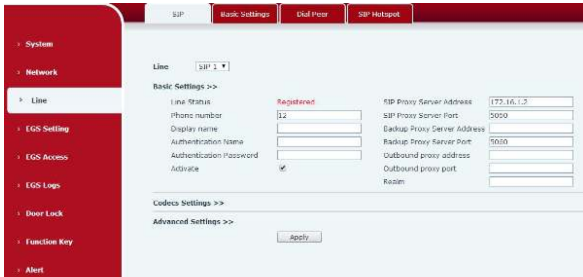
Figure 4 - SIP Line Configuration
